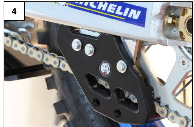
Place the Th 6x60mm + Th 6x15mm Placer les Th6x60mm + Th 6x15mm
