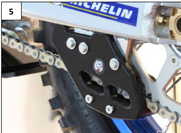
Place the Tfhc 6x60mm Placer les Tfhc 6x60mm
