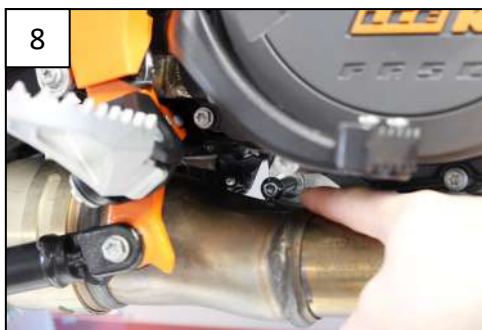
4 Position the clamped bolts as shown (4) and push them to the bottom (5)
