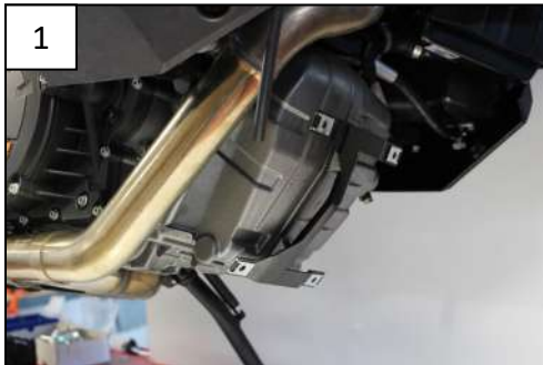
1 Remove the OEM skid plate and keep the front fixation
