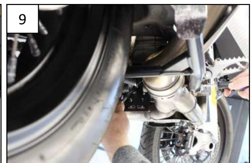
6 Prepare step (7) with Tbhcs 8x50mm + 2 M8 Washers + 1 Em8f
