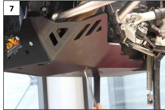
7 Place the 3 Tbhsc 8x50mm screws in the middle of the skid plate with M8 Washers and tight everything
