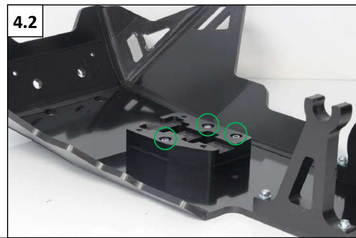
4.2 Fix the plastic block on the skid plate with 3 Tfhc 6x40mm + 3 Em6f + 3 M6 Washers
