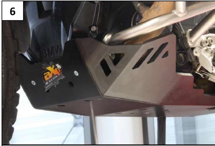
6 Place the front Tbhsc 8x35mm screws with M8 Washers
