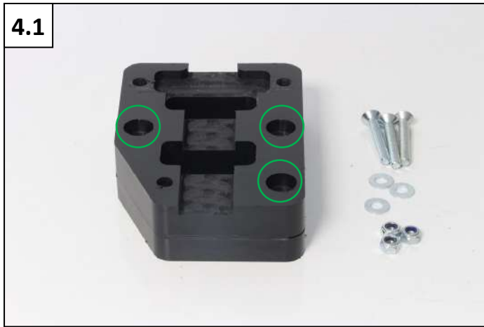
4.1 Fix the plastic block on the skid plate with 3 Tfhc 6x40mm + 3 Em6f + 3 M6 Washers
