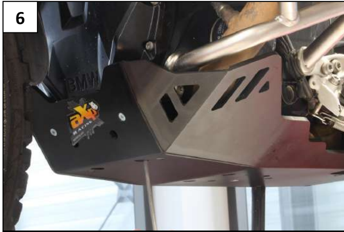
6 Place the front Tbhc 8x35mm screws with M8 Washers
