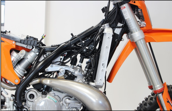
Start by removing the tank and the plastics (1) . Fix the 128mm spacers on both alloy small parts (2)
