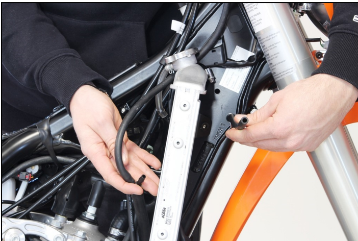
You can remove the cables (3) to make a good fitting (4). Use the windows done to make the cables passing
