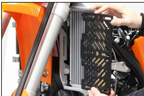
For right and left sides, place the grids, fix it with Tbhc 6x20mm and M6 Washers (13) (14). Finally, put the tank in place and fit everything (15)
