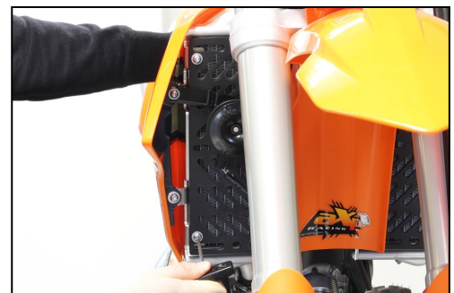
For right and left sides, place the grids, fix it with Tbhc 6x20mm and M6 Washers (13) (14). Finally, put the tank in place and fit everything (15)
