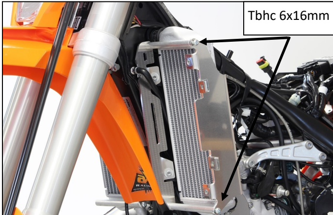
Place the biggest parts of the kit on left and right sides considering the Fan will go on the right (10) (sitted on the bike). Position the screws without tightening anything
