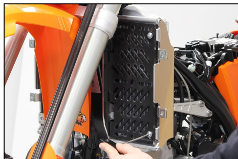
For right and left sides, place the grids, fix it with Tbhc 6x20mm and M6 Washers (13) (14). Finally, put the tank in place and fit everything (15)
