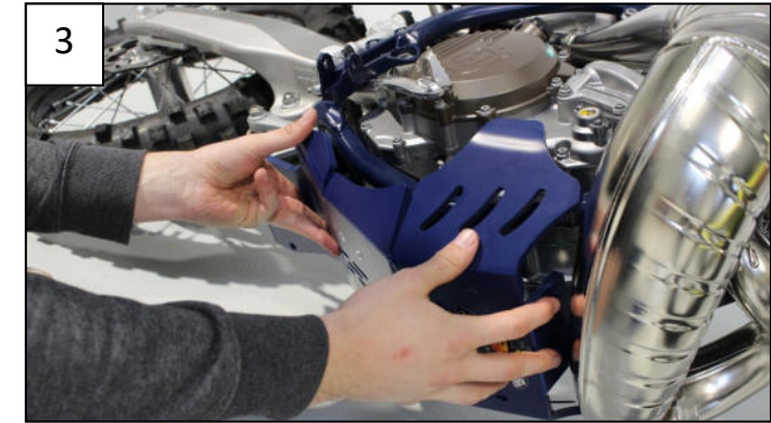
Clip the rear of the skid plate on the rear tube
