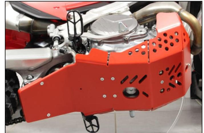
You can drain oil without removing the plate
