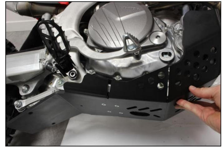
Push the skid plate in direction of the engine and then slide it to the rear to position the rear mounts on the rear frame tube
