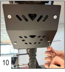
Lift the plate up and tighten the four 6x25 screws.
