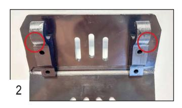
Place the rear hooks with the machined faces on the outside.
