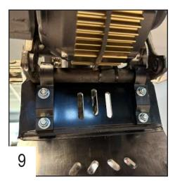
Insert the plate on the frame using the 2 hooks.
