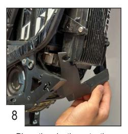
Place the plastic protection back and fix the second front fixation on the left side.
