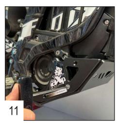
Place the stickers and fix the cover using the three 6x16 screws. Repeat the operation on the other side.
