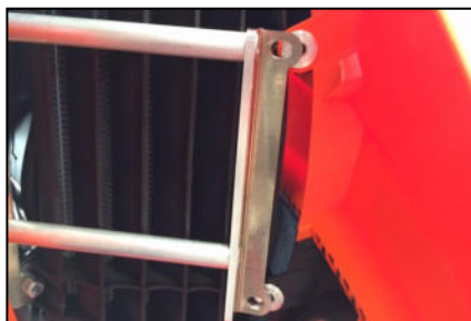
Put the plastic between the bloc and the air deflector
