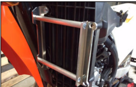
Fix the bloc with Tbhc 6x16 + R.M6 on the air deflector points
