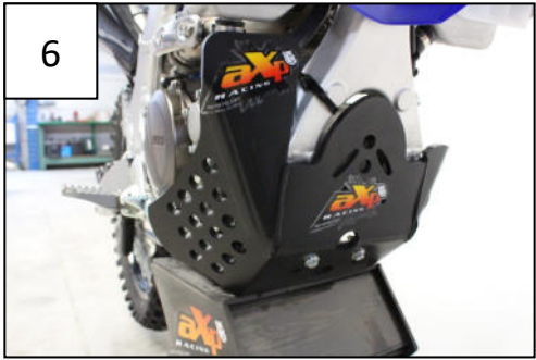
Intsall the front bracket PM02-07-008 + Clamped bolt
