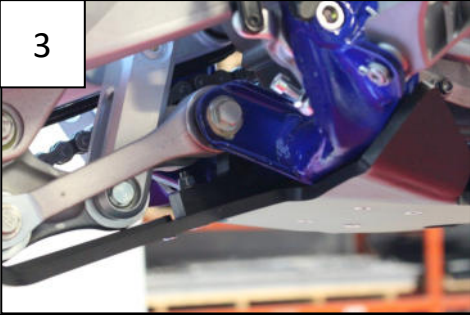
Clip and fit the skid plate to the rear tube
