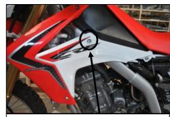
Put back the platic with original scres except 1 Tbhc6x20 + R.M6 as indicated
