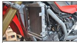
Fix the kit on the radiator with original screws
